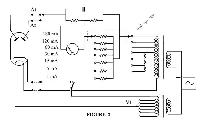
taken in order and all the others strapped together. The denomination of the electrodes between which any breakdown exists will thus be automatically indicated and further, the continuity of the heater circuit is shown as a zero resistance at the heater (**H**) position of the switch.
