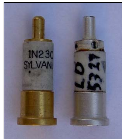
Design differences between the military diodes of Sylvania and Western Electric. LHS-sectional view (image from [RIO 97]), RHS photo of the Sylvania 1N23C and the Western Electric 1N21 (Author's Collection)
