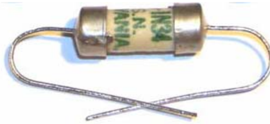
The First US Commercial Diode, the Sylvania 1N34 [WAR]
