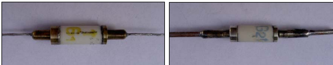
Left: yellow type C WG1 diode and right: blue WG2 cartridge (with added leads) (Author's collection)
