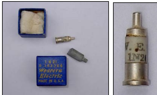
Western Electric 1N21 diode February 17 th 1944. Note the protective lead capsule. Western Electric was the commercialization company of Bell Laboratories (Author's Collection)
