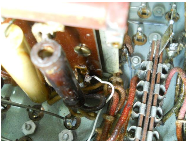
Figure 8. Connecting the 12.6 VAC supply
