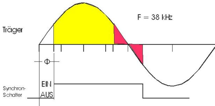
$$U_a = U_s \int_{\varphi}^{\varphi+180} \sin(\alpha) d\alpha = U_s * (-\cos(\varphi+180) + \cos(\varphi))$$
