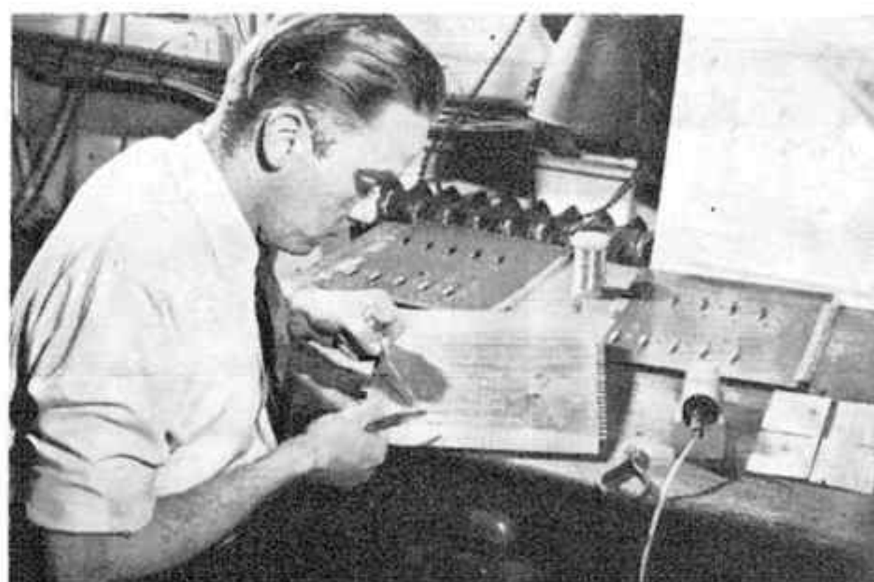
Printed wiring boards are equipped by hand. Terminals at end permit rewiring to provide other counter and storage facilities
