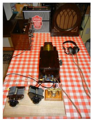
Ham radio equipment ground. The signal in the headphones is barely audible in this case, but a strong signal is obtained in the vintage high impedance speaker, with little distortions. When this vintage amplifier is replaced by a modern guitar amplifier the sound quality is exceptional, as in the headphones.
